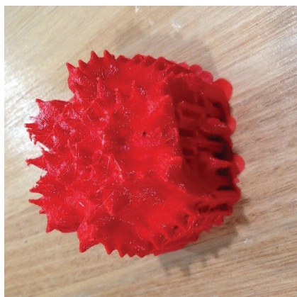
Figure 5 a and b: Initial print of Microseris lanceolata with structures in place (left) and with structures removed (right).
